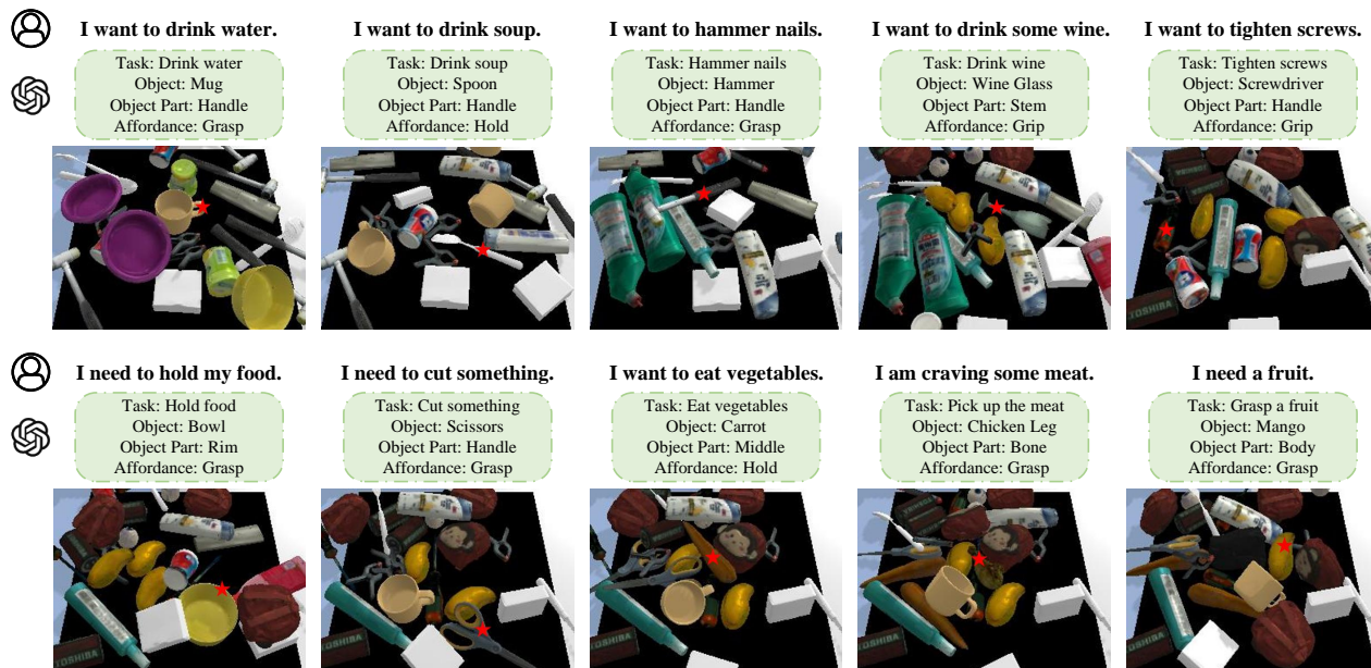
Fig. 4. Simulation Cases of Grasping in Clutter: The affordances of the target object are indicated with red stars.
